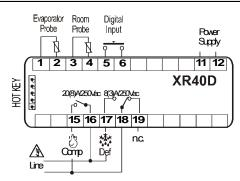
24Vac/dc supply: connect to the terminals 11 and 12. 120Vac supply: connect to the terminals 11 and 12. 230Vac supply: connect to the terminals 11 and 12.
